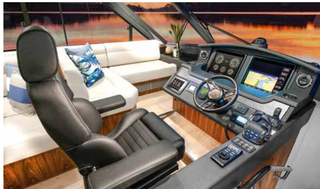
Skippers will be right at home at the helm, which utilises Volvo Penta's touchscreen Glass Cockpit technology.
